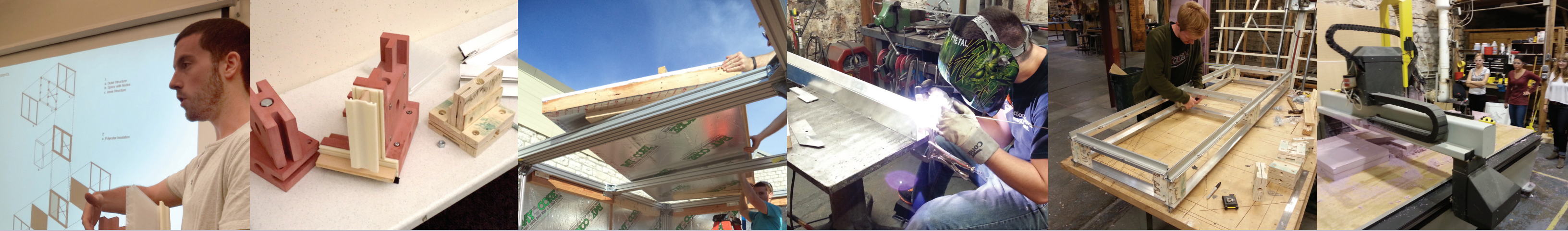
(left to right): Students (Brian Conklin pictured) proposed and developed new curtain wall systems in the studio, emphasizing the relationship between materials, assemblies, and energy performance; to improve the curtain wall, the system developed by Brian Conklin, Dylan Rupar, and Nick Nelson used a double skin and connection nodes shown above as process models; students built a reusable testing enclosure, supported by NCARB Award funding, to test their curtain wall prototypes at full scale.
