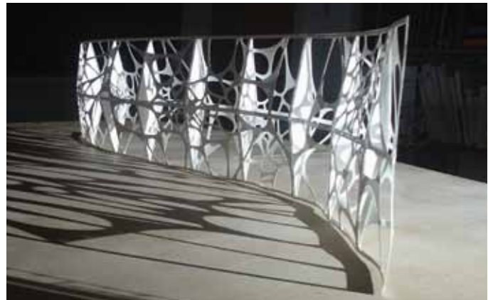
Figure 4. Three-quarter inch scale prototype with solid vertical fins.
