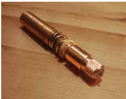
Figure 7. This is the die cutting device fabricated to fit in the routers 1/2-in. collet along with a compression added to allow for exact pressure to be applied during cutting.
