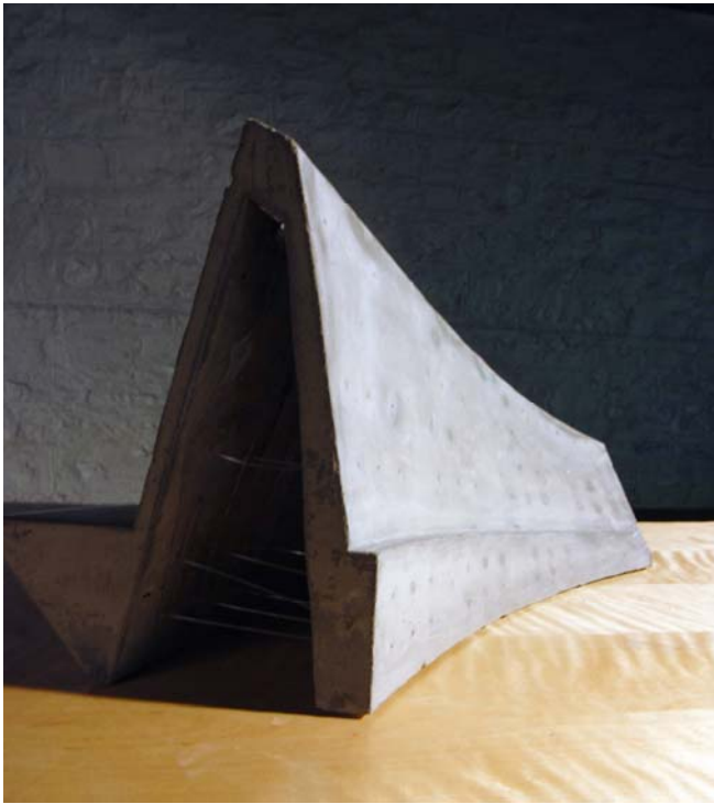
Figure 6. This model tests the tie rod pattern. Acrylic rods hold the acrylic sheet in equilibrium during the concrete pour.
