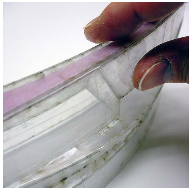
Figure 3: Fabricated using a CNC laser cutter, this ¾" scale acrylic model represents a complete formwork for a concrete pour.
